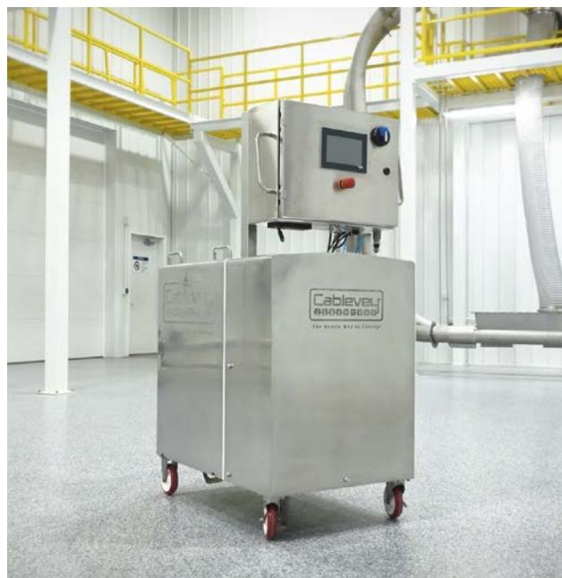
Cablevey Smart Cart mid-room: The cart is specifically designed to be a fraction of the size of similar carts on the market to facilitate mobility.
