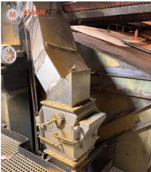
Dual Round Nose Plate Magnet in a rendering application
