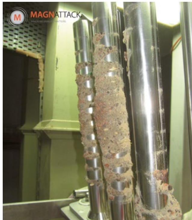
Contamination collected on Rapidclean® Bars
