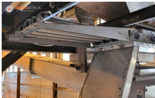
Mag-Ram® Self-Cleaning Magnet in meat rendering
